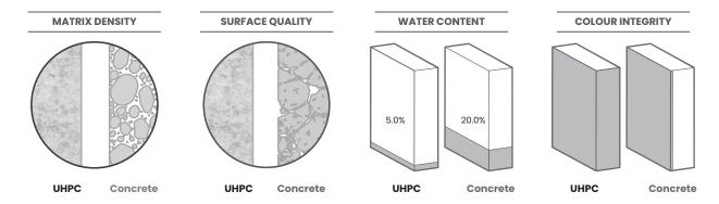
High packing density yields excellent flexural strength that is over four times higher than regular concrete.
